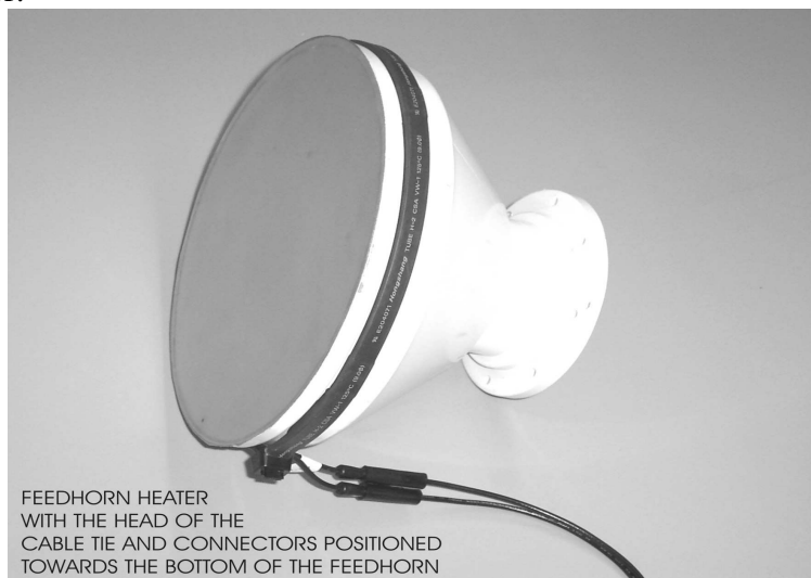
Feedhorn Heater Placement
